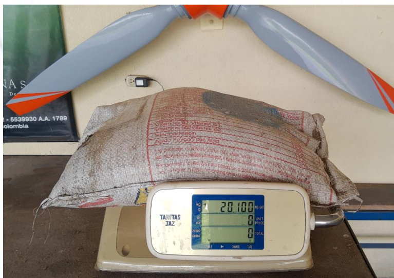
Figure 3. Sample of a 20kg sandbag used as deadweight.
