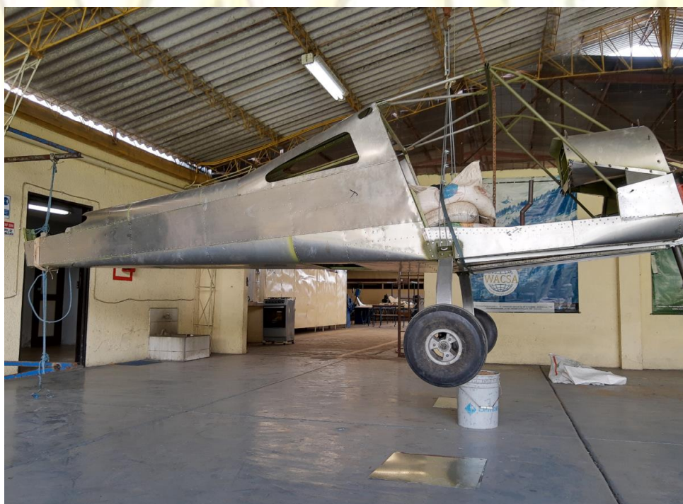
Figure 14. Aircraft raised at required height of 0.41m (41cm)
