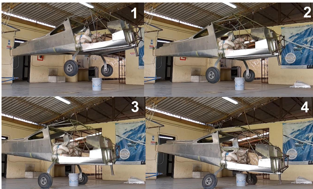
Figure 15. Sequence shot of the drop test. From highest height to the position of maximum deflection (Side view)
