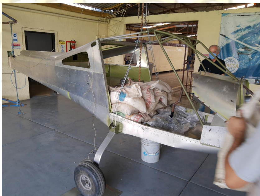
Figure 10. Process of weighing and loading the aircraft
