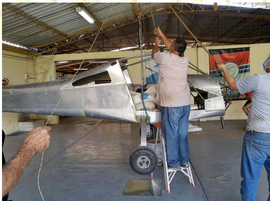
Figure 12. Process of lifting the aircraft
