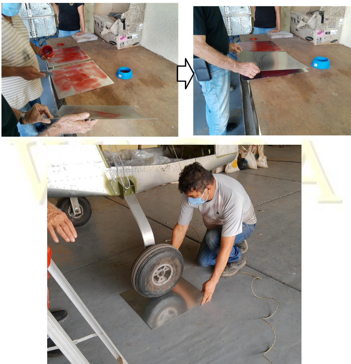
Figure 6. Lubricated plates under the wheels
