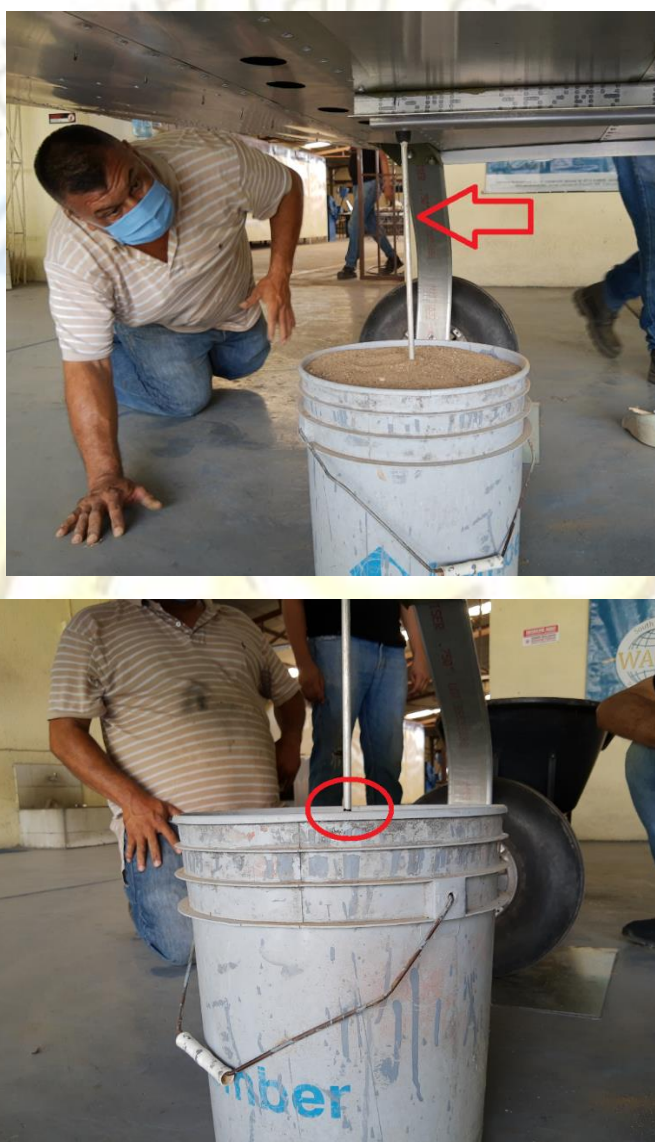
Figure 7. Stick and its zero reference mark employed to measure vertical deflections
