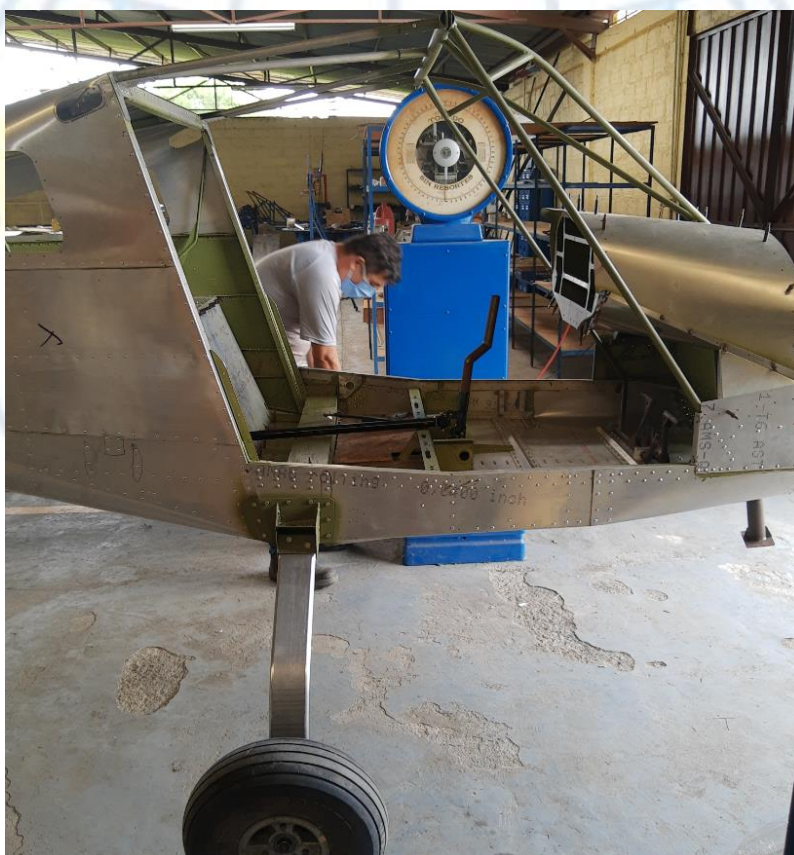
Figure 1. Aircraft structure weighing procedure
