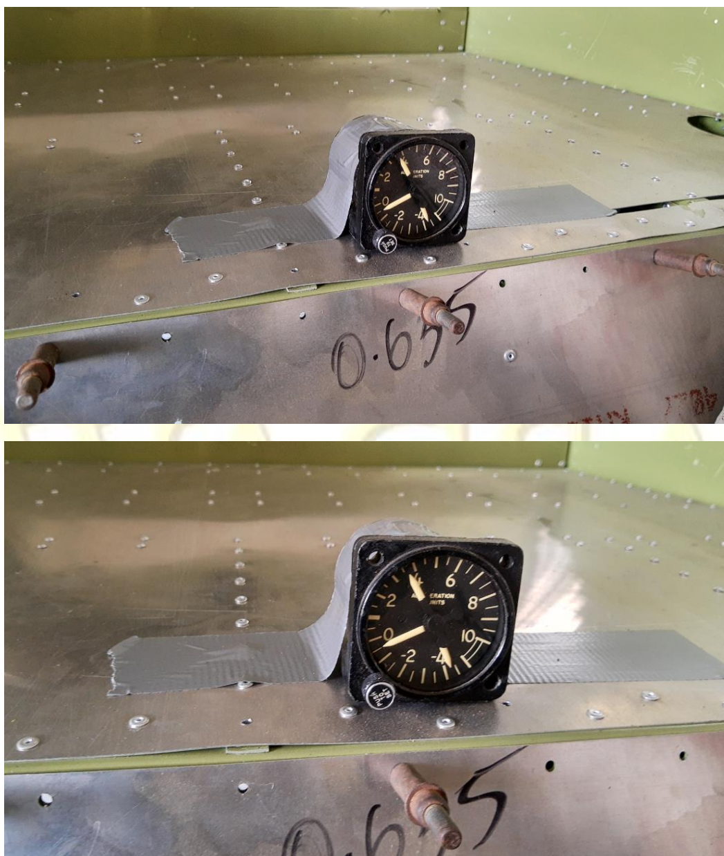
Figure 20. Maximum vertical deflection measured
