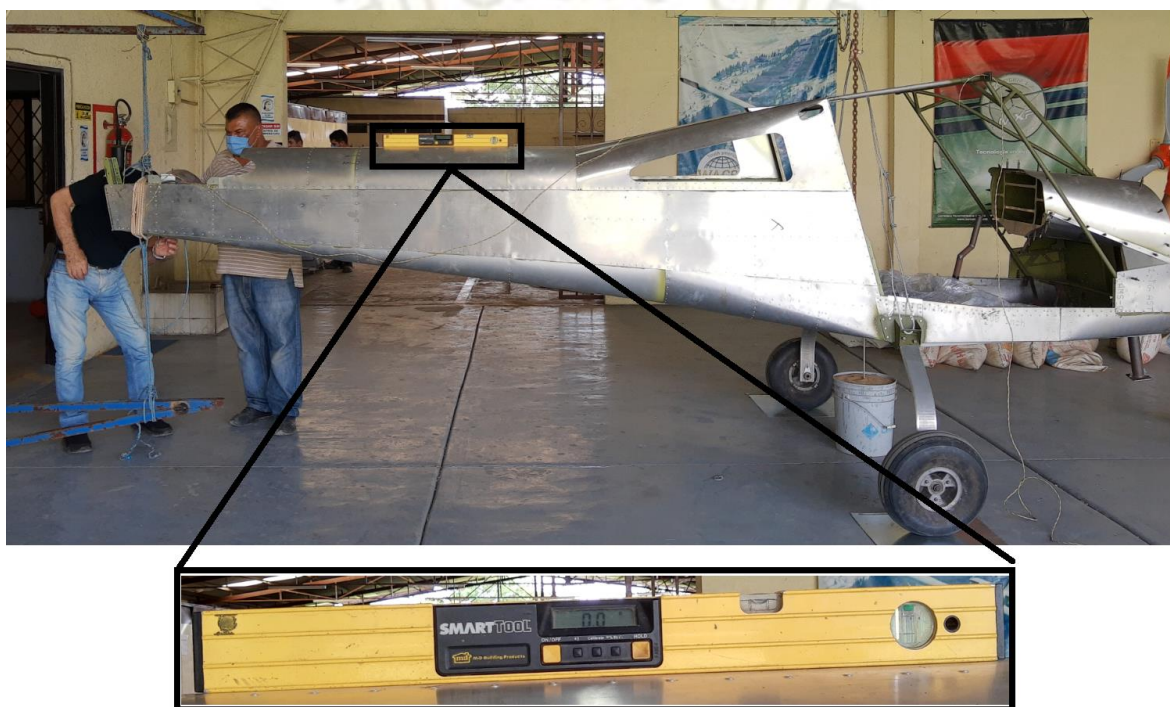
Figure 4. Aircraft position when touching the ground (level)
