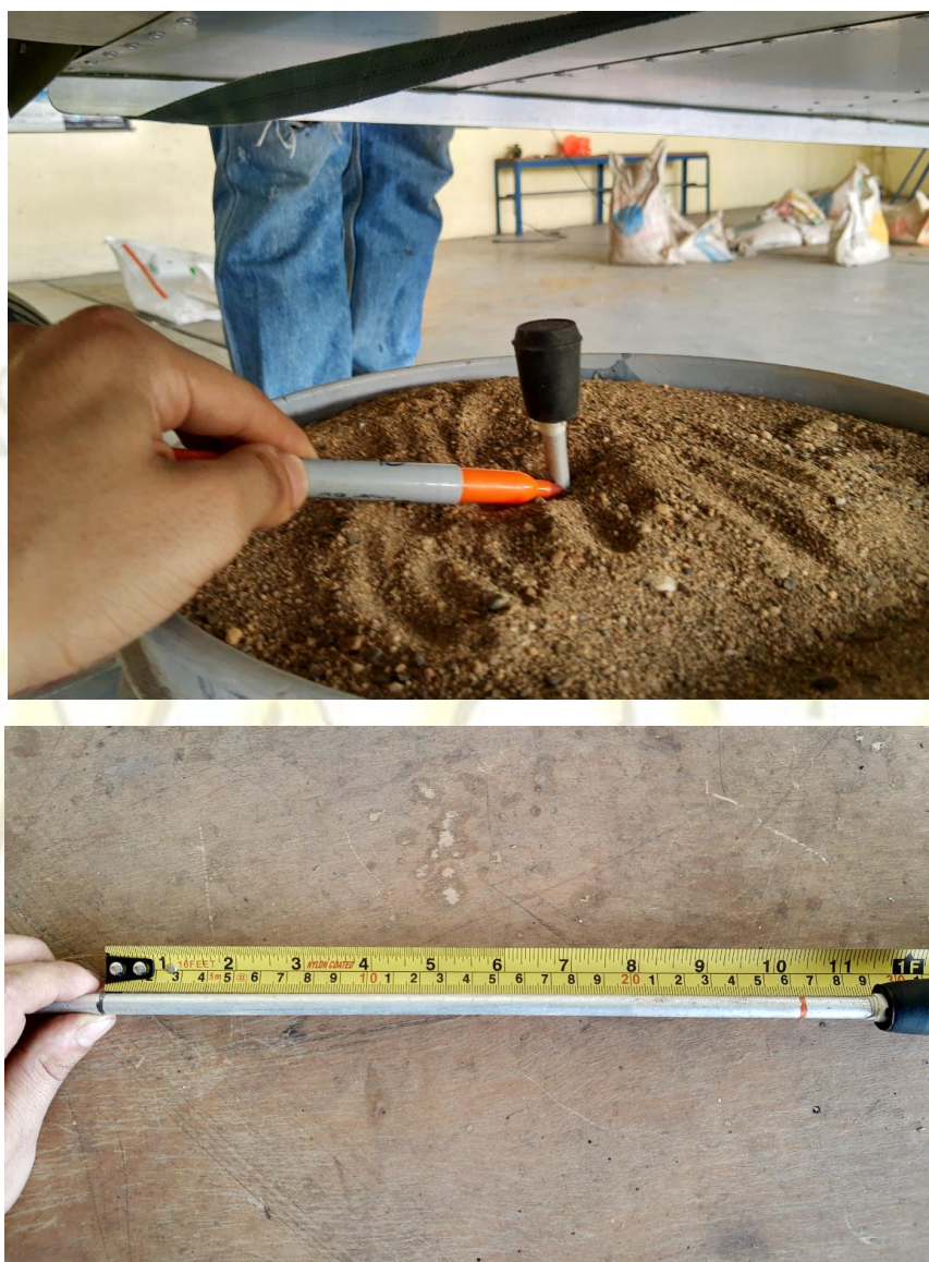
Figure 19. Maximum vertical deflection measured (0.265m)
