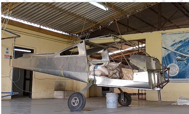
Figure 16. Final position after the drop (Side View)
