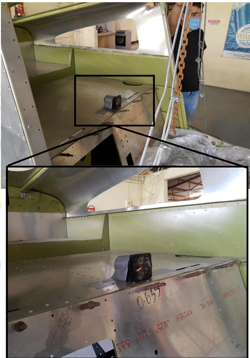
Figure 8. G-meter used to register accelerations
