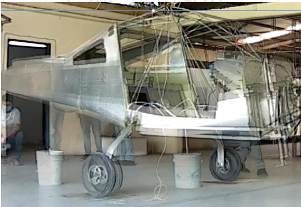
Figure 21. Overlapping image showing the settling deformation of the brand new landing gear system (before and after the test)
