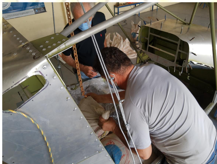
Figure 9. Process of weighing and loading the aircraft
