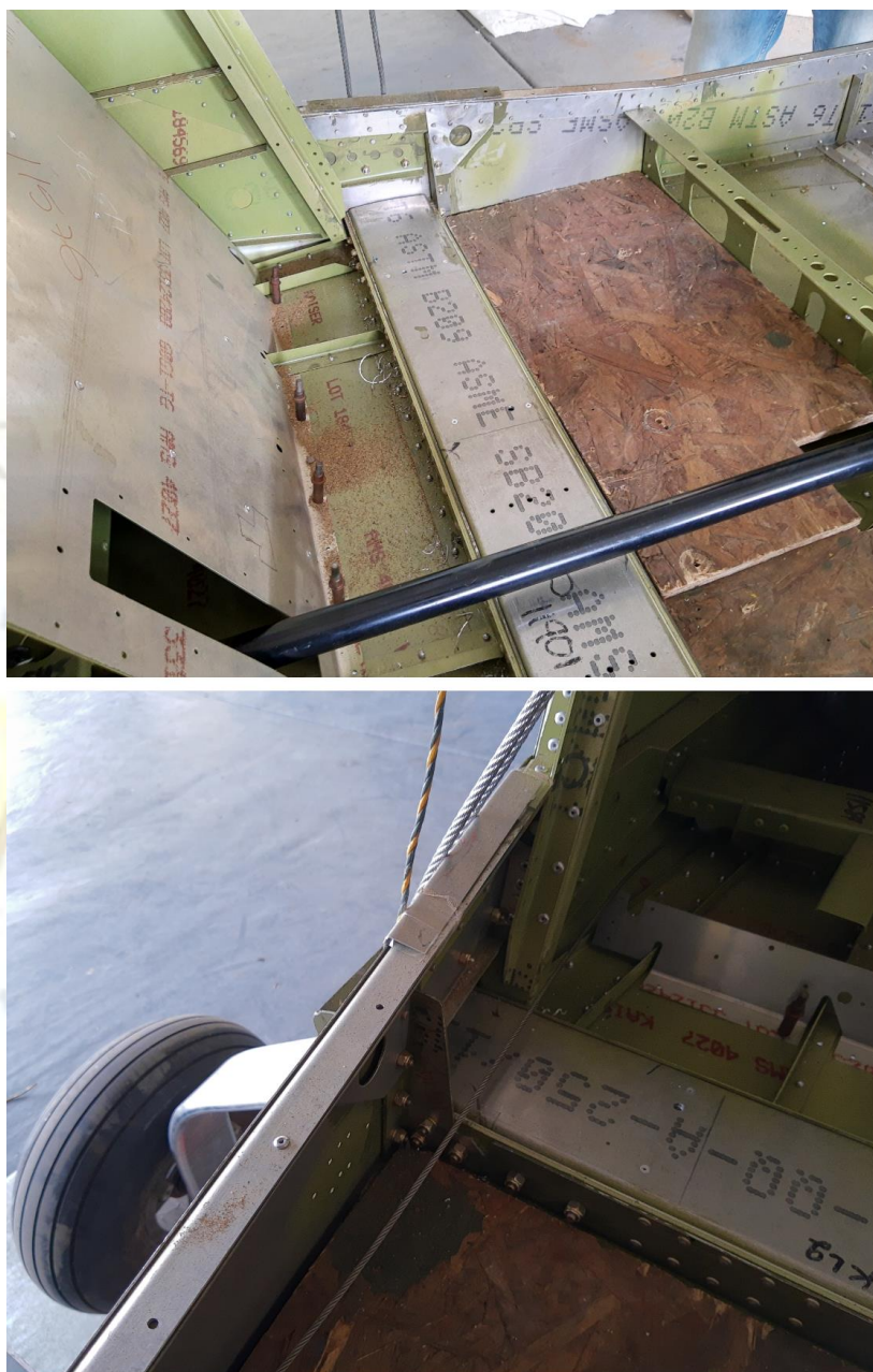
Figure 22. Both left and right internal side as well as all surrounding structure remained intact after the test
